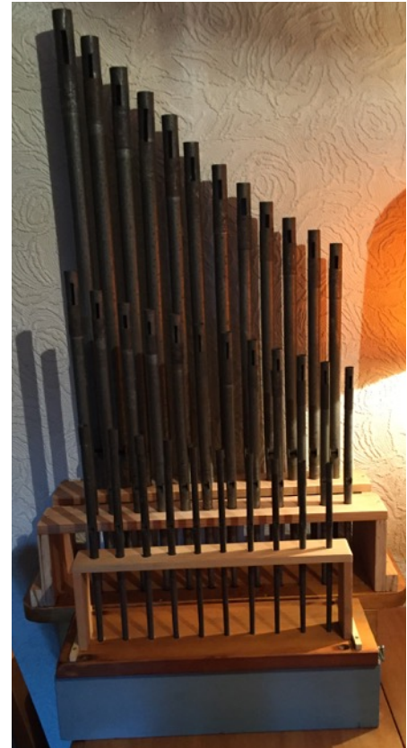
Top two Gamba chests with pipe racks and pipes
