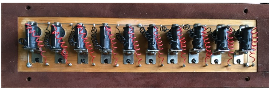
Magnets attached to the topboard, inside top Gamba wind chest
